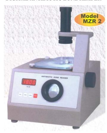
The antibiotic zone provides a rapid accurate method for determining the strength of antibiotic materials by measuring the diameter of an inhibited zone in Petri- dish
